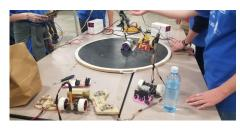
The Mini-Sumo Robot is an of internationally standardized class which robotic competition, has traditionally seen most competitions use a computer-programmed chip to control the robot.
